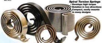
Spiral torsion springs are normally used in applications requiring less than 360 degrees of rotation. They are generally used to obtain a large amount of torque through a small amount of rotation. (continued on back)
